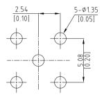
RECOMMENDED PCB MOUNTING HOLE LAYOUT
